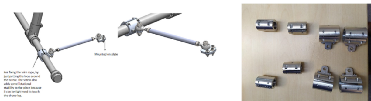
Fig. 4.9: (Left) Detail of the attachment of the systems' mounting plate onto the drone's landing gear. (Right) Manufactured mounting clamps out of aluminum.
