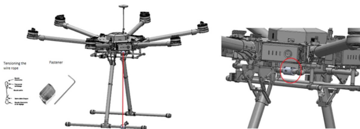
Fig. 4.8: Drone CAD and mounting equipment sketch for supporting a plate where all emission monitoring systems will be attached. Red line on the left shows the position of a wire rope supporting the drone's landing gear. The red circle on the right shows an in-house clamp where the wire rope will be attached.
