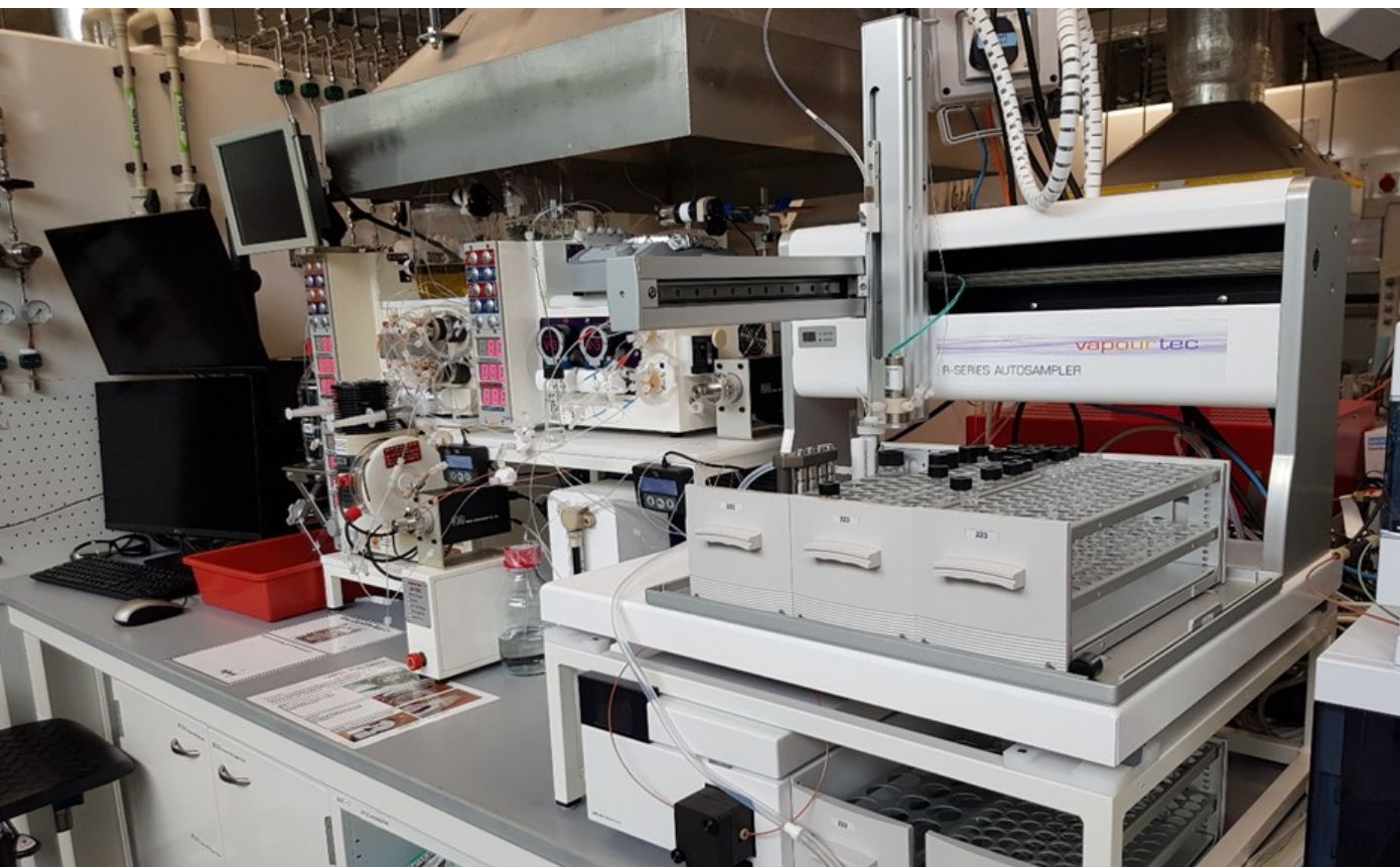
Fig. 1: Chemical handling equipment and reactors for automated optimisation.
