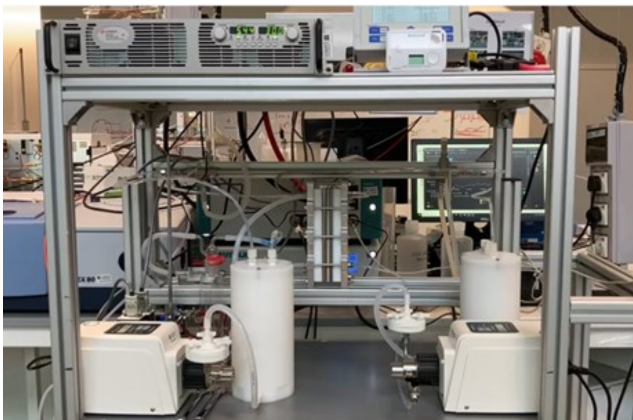
Figure 8.2: Table top chemical reactor constructed in eCO 2 EP for the conversion of CO 2 to value-added chemicals.
