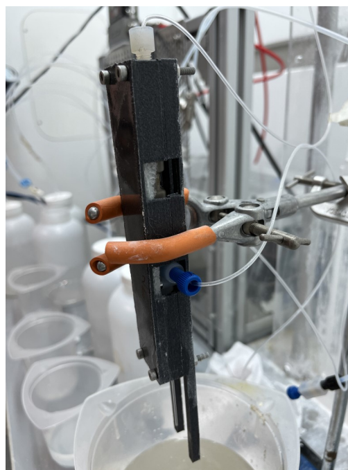
Figure 1.5: 1kg scale ZnO synthesis using annual flow microreactor
