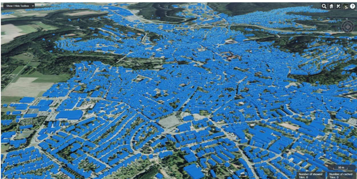
Figure 8.10 Visualisation of exported models of Pirmasens building data on the 3DCityDB-Web-Map-Client.
