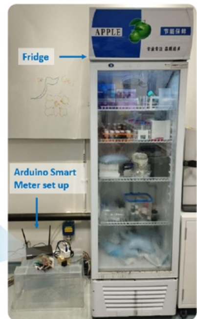
Figure 6.1: Smart meter prototype to measure the electricity consumption of a fridge in the CARES Laboratory, and the temperature and humidity of the surroundings.
