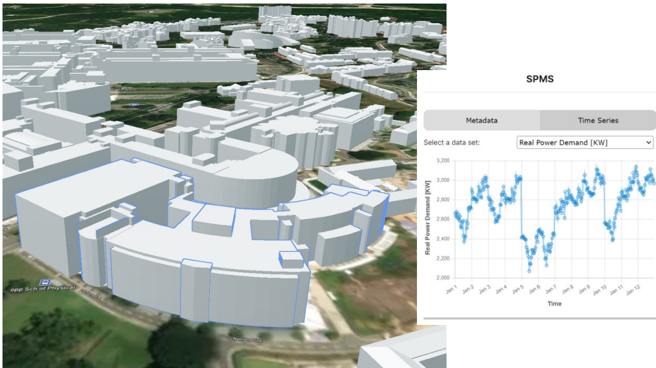
Figure 9.2: Visualisation of the instantiated buildings on the NTU campus displaying historical power consumption data for the School of Physical and Mathematical Sciences (SPMS) building.
