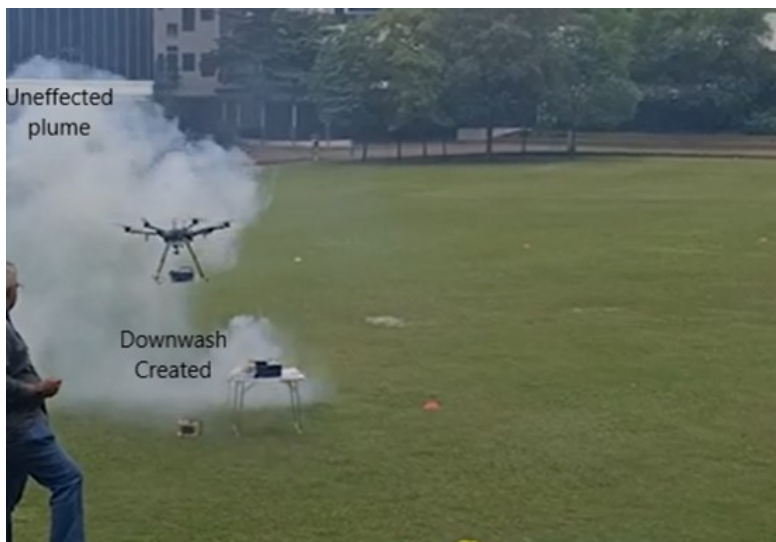
Figure 4.10: Drone demonstration outside of CREATE Tower showing the influence of the unmanned aerial vehicle (UAV) on the plume it is sampling. Here, the payload is fitted for particle detection.
