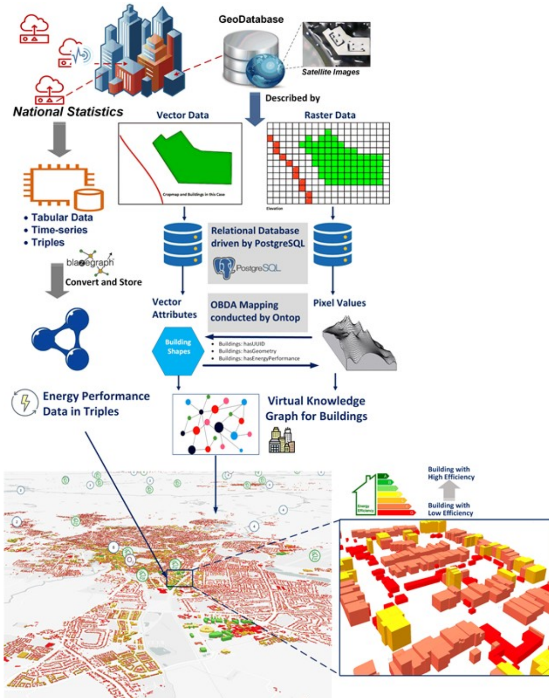
Figure 5.10: Workflow for integrating geospatial descriptions of buildings and their energy performance using the World Avatar dynamic knowledge graph.
