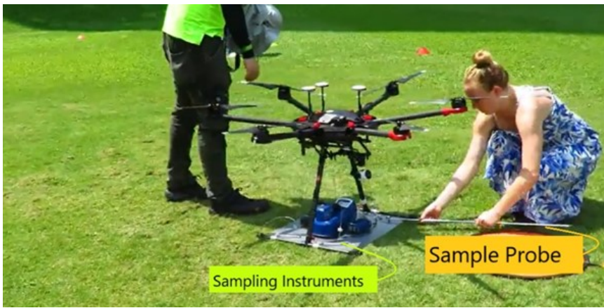
Figure 4.11: The Sample Probe protrudes 90 cm from the UAV’s center, enabling sampling from outside the UAV’s downwash. The sampling instruments are also shown. Here, the UAV is equipped with particle instruments.
