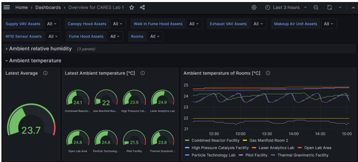
Figure 5.11: An analytical dashboard displaying the ambient temperature for various rooms in the CARES laboratory.
