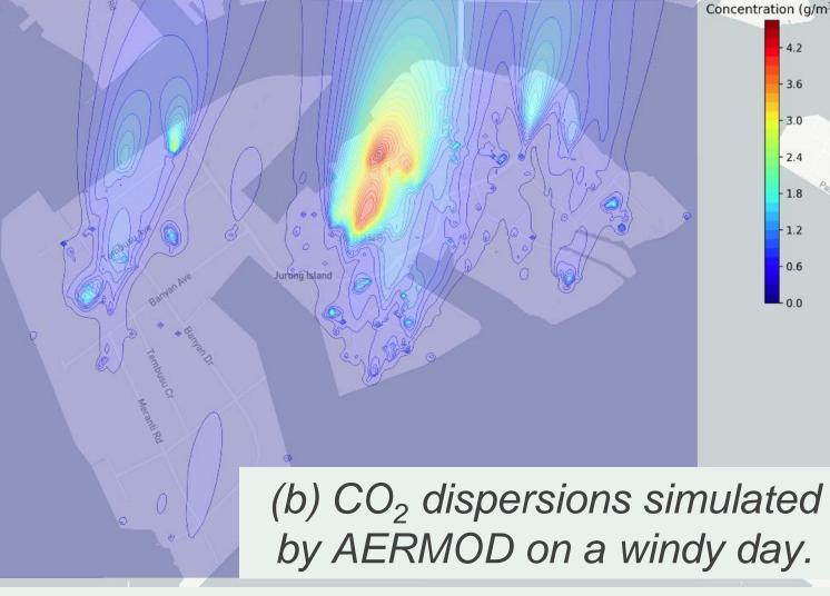
Figure 2. CO<sub>2</sub> dispersions on Jurong Island simulated by AERMOD during different weather.
