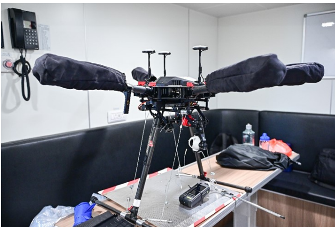
Figure 4.1 (a): CARES's drone with attached payload (methanol and ammonia sensors).
