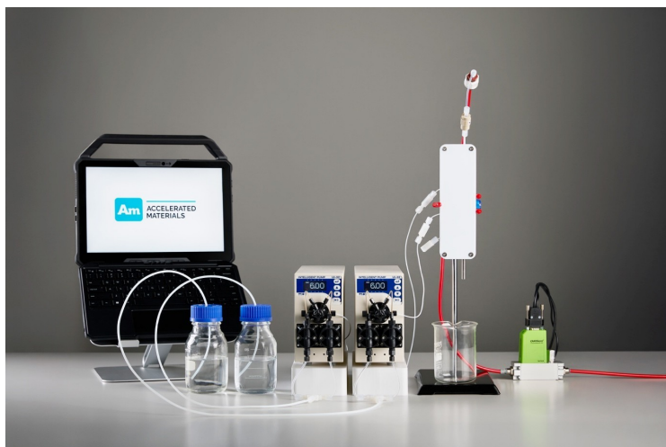
The reactor built in the CARES laboratory to scale up nanomaterials.
